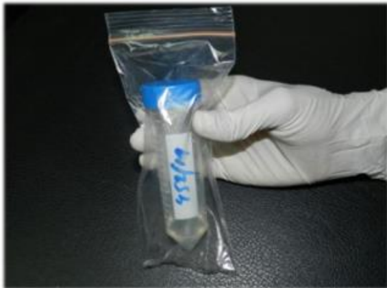
Figure 4: Insert the tube to the Zip lock poly bag and close properly
